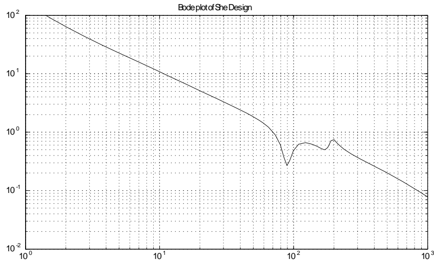
Figure 10: Frequency response of the loop gain in the referenced paper
