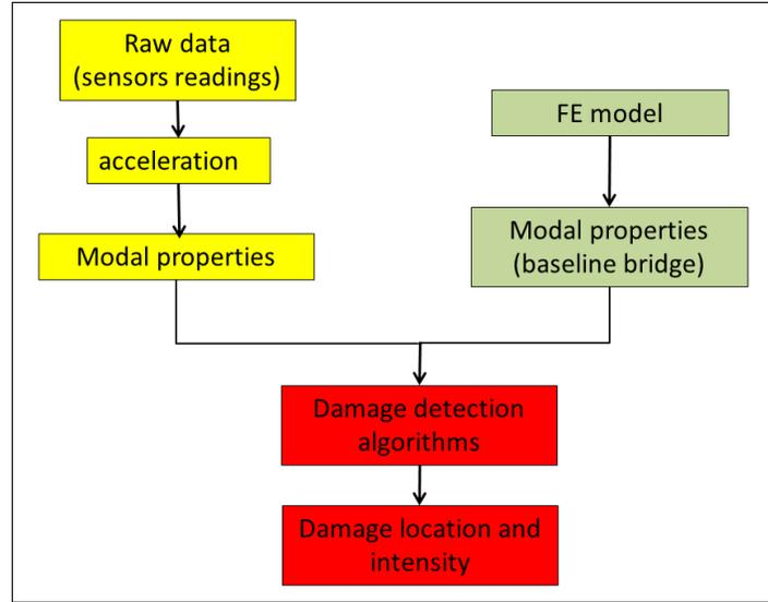
Figure 4-1: Damage detection procedure
