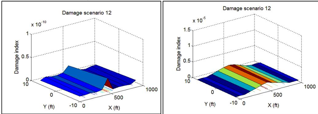
**Uniform load surface curvature method**
