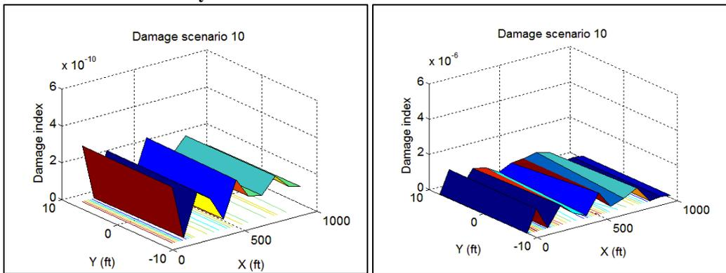
**Uniform load surface curvature method**
