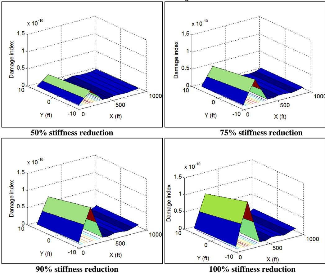
Figure 6-7: Results for damage scenario D1 (different damage intensities)
