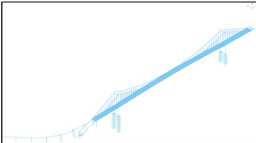
Figure 2-2. Finite Element Model of the Alfred Zampa Memorial Bridge
