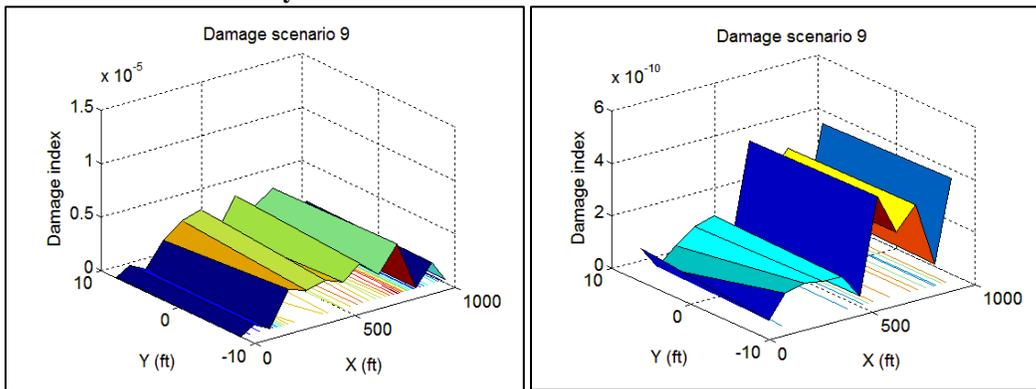
**Uniform load surface curvature method**
